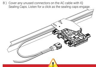
WARNING: Install sealing caps on all unused AC connectors as these connectors become live when the system is energized. ealing caps are required for protection against moisture ingress
