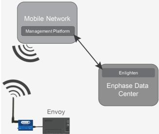
The Envoy connects to the modem using a USB cable. The USB cable also powers the modem.
