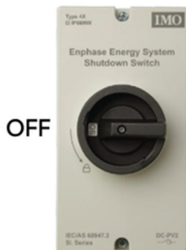
Figure 6 : Correct position of rapid shutdown switch before powering IQ System Controller 2
