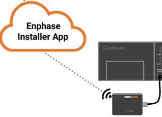
The Enphase Mobile Connect is a modem package that connects to the Enphase Envoy-S or IQ Gateway, and eliminates the need for an on-site Internet connection to monitor an Enphase Microinverter System. The addition of The Enphase Mobile Connect to an Enphase System enables greater installation flexibility and provides reliable system monitoring independent of the Internet service on site.
