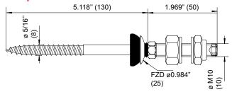
7.3 inches EJOT Solar Fastening System for wood substructure
