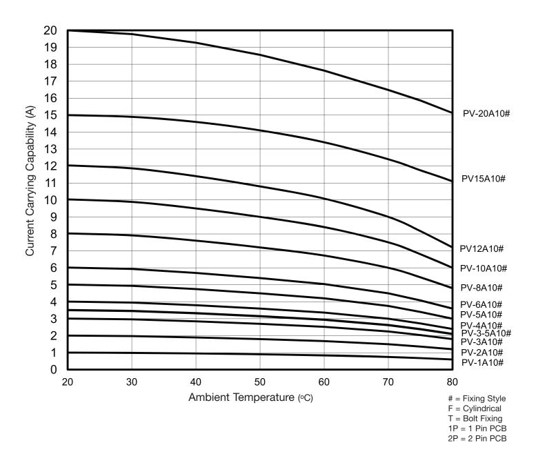
No additional derating is required for PV fuse links installed in ganged modular fuse holders without spacing between units, provided that the rating used is  $>1.56 \times I_{sc}$ .
