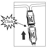
Best Practice: Use the Bus Cable Unlock Tool of AC Bus to split the connectors.
