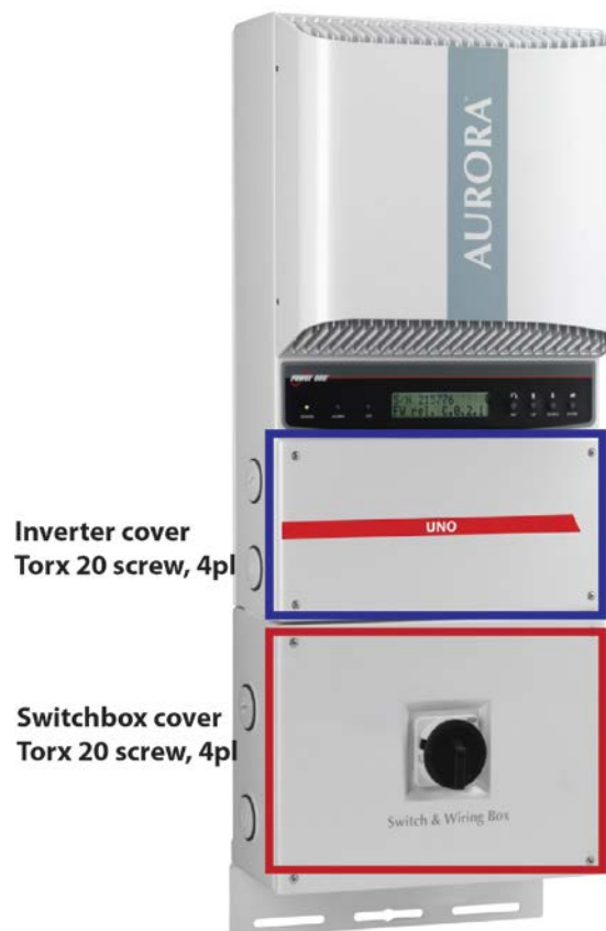
Figure 3-2: Front Access Panel Location
