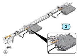
USE RACKING SYSTEM CERTIFIED FOR USE AS A GROUNDING STRUCTURE.
