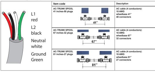
The installation technician is responsible for selecting a junction box with the appropriate dimensions and insulation. Do not reverse the phase and the neutral!
